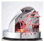
The PATLITE LED revolving warning light uses a unique and patented reflecting system, solely designed for these models. Even though the dispersion characteristics of the LED chip is less than an incandescent bulb, PATLITE's unique design creates an equivalent dispersion effect with the light reflector.
